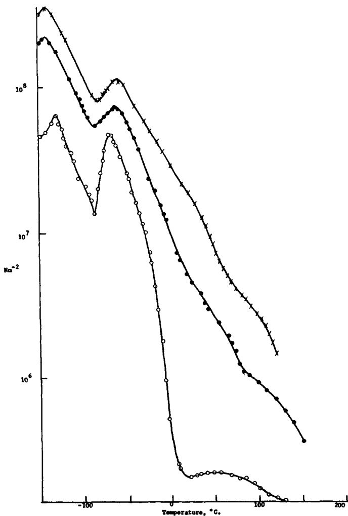
Fig. 7. Loss modulus ( E'' ) vs. temperature for Lycra at 110 Hz and 2% (O), 200% (●) and 400% (×) static strain.
